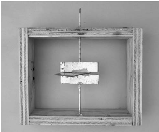
Fig. 3 Aluminum phantom model mounted in wood frame
