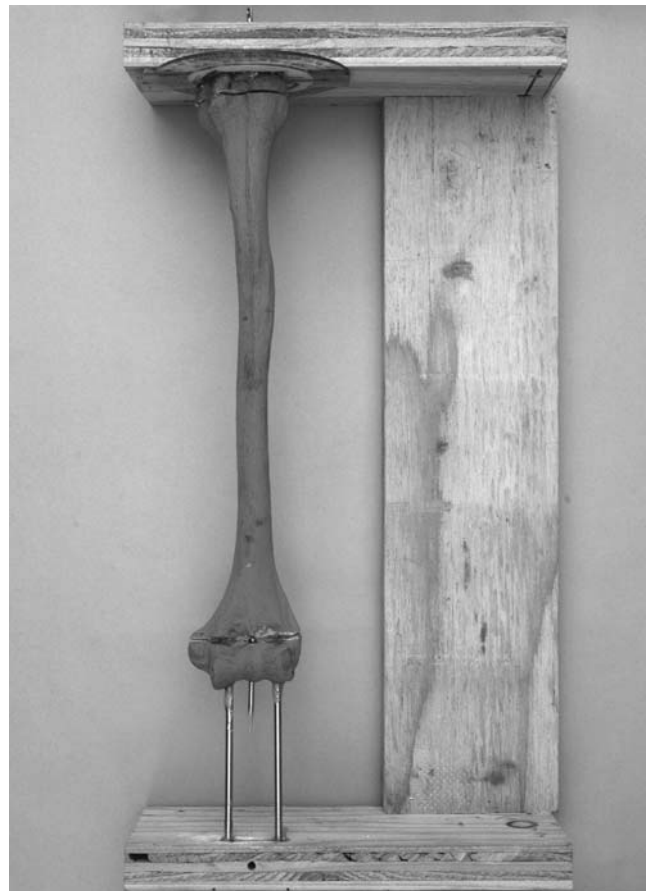
Fig. 2 Pediatric supracondylar humerus fracture model mounted in wood frame
